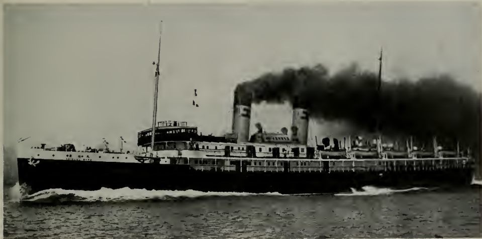
Keifuku Maru is operating as a passenger and cargo vessel, gross tonnage is 5833, net tonnage 4241. She was built in 1919 at the Kawasaki shipyard, Kobe, for the Daiko Syosen K. K. Her length is 385, beam 51, depth 36 and her speed is 10 knots.
